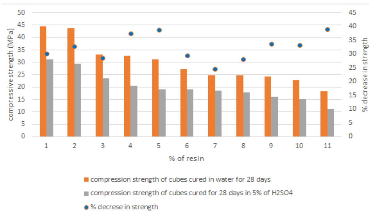
Fig. 13: Comparison of Compressive Strengths of normal concrete cubes and cubes cured in 2.5% H 2 SO 4 solution
